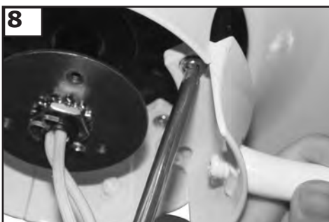
8 Remove 2 screws per blade holder. Remove blade holder. When replacing blade holders make sure the screws are tightened securely to the motor.
