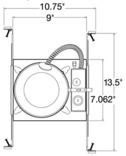
Non-IC Light 6" Housing for New Construction
